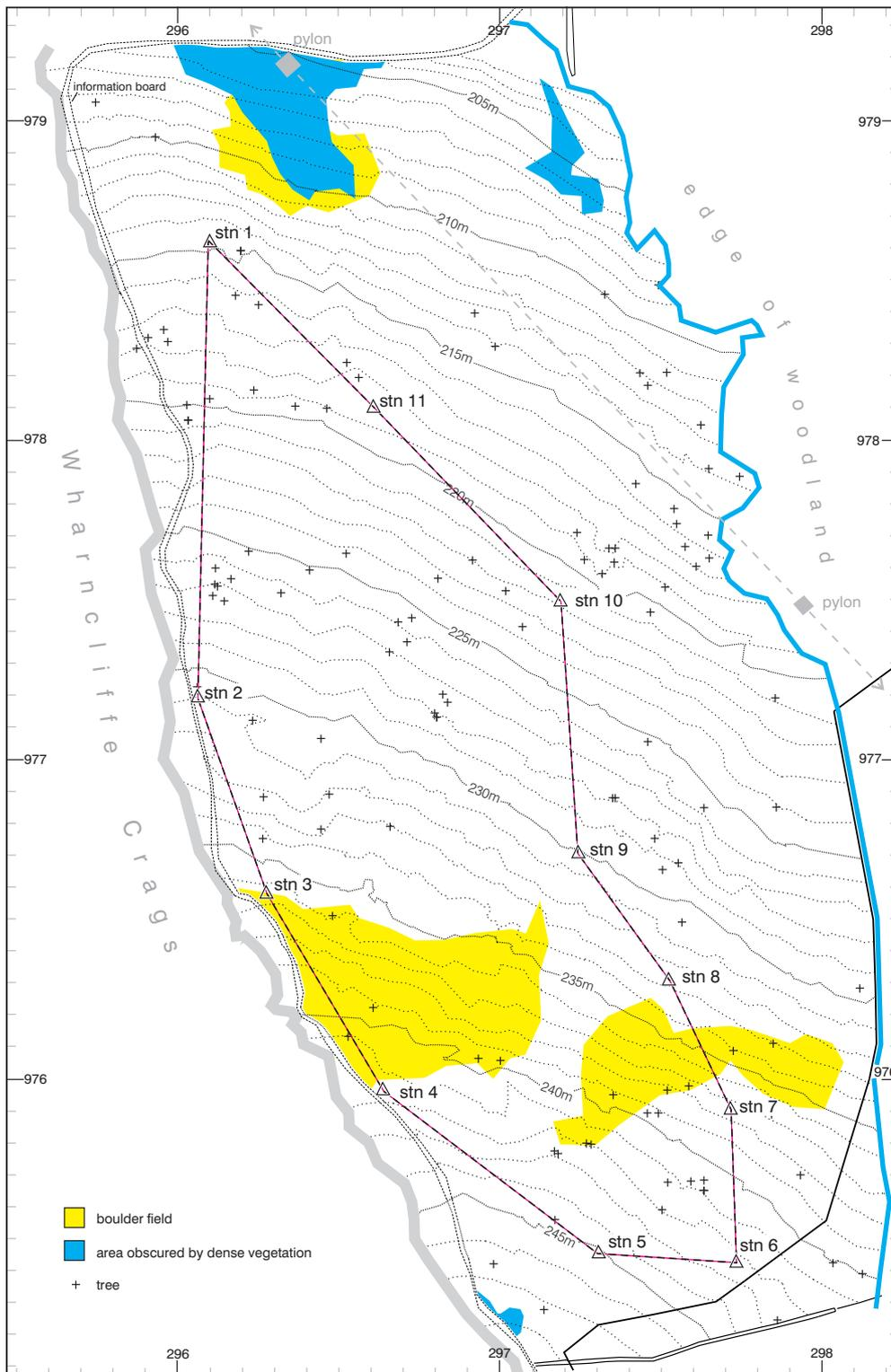
Figure 22. Survey traverse showing location of survey stations (stn 1-11)
